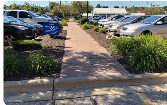
Parking medians and islands with walking paths offer pedestrians a safer, separated route away from vehicles.
